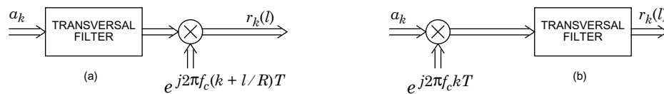
Fig. 20-8. Two configurations for one interleaved echo canceler corresponding to a passband channel. a. A baseband transversal filter followed by modulator. b. A modulator followed by a passband transversal filter.
