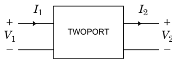
Fig. 18-7. Illustration of a twoport network with definition of voltages and currents for the chain matrix.
