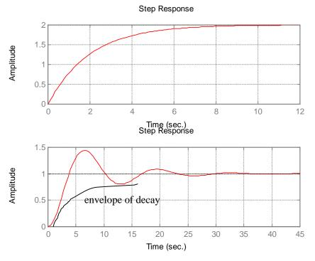
First order system (top plot) has general form  $H(s) = \frac{k}{s+a}$ . The time-constant is the time that the response is equal to  $2(1-e^{-1}) = 63\%$  of 2 = 1.26, so  $\tau \approx 2$  sec.  $a=1/\tau = 0.5$ . The steady-state value (due to a unit step input) is H(0) = k/a = k/0.5. From the plot 2 = k/0.5 so k = 1.
