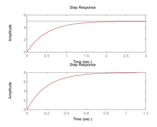
f) The actual closed loop system is represented by  $G_{cl}'(s) = \frac{G_c G_p'}{1 + G_c G_p} = \frac{K_P}{1 + K_P + 0.5}$
