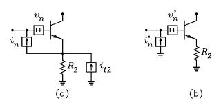
3. The figure shows the ac signal circuits for single stage CE and CB amplifiers. The transistor parameters are  $\beta = 100$ ,  $r_x = 40\,\Omega$ ,  $r_0 = 50\,\mathrm{k}\Omega$ , and  $V_T = 25\,\mathrm{mV}$ . (The formulas for the voltage gain, input resistance, and output resistance of the CE and CB amplifiers are given in Section 7.6 of the class notes. You do not have to derive these.)
