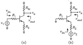
(a) For the CE amplifier of Fig. (a), it is given that  $R_1 = 1 \,\mathrm{k}\Omega$ ,  $R_2 = 50 \,\Omega$ , and  $R_{tc} = 10 \,\mathrm{k}\Omega$ . Show that  $I_{C(opt)} = 228 \,\mu\mathrm{A}$ . For  $I_C = I_{C(opt)}$ , show that  $v_o/v_1 = -51.4$ ,  $r_{in} = 16.2 \,\mathrm{k}\Omega$ ,  $r_{out} = 8.76 \,\mathrm{k}\Omega$ ,  $v_{ni}/\sqrt{\Delta f} = 4.4 \,\mathrm{nV}/\sqrt{\mathrm{Hz}}$ , F = 1.21, and  $NF = 0.829 \,\mathrm{dB}$ .
