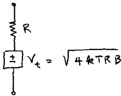
where we have used a square symbol for a noise source. The polarity of the source is arbitrary. The Thévenin circuit can be converted into a Norton circuit. The Norton current is given by
