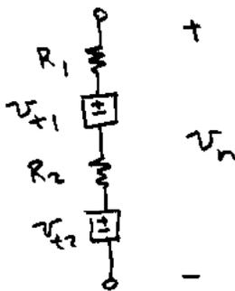
$$\begin{aligned} \overline{v_n^2} &= \overline{(v_{n1} + v_{n2})^2} \\ &= \overline{v_{n1}^2} + \overline{v_{n2}^2} \\ &= 4kTR_1B + 4kTR_2B \\ &= 4kT(R_1 + R_2)B \end{aligned}$$
