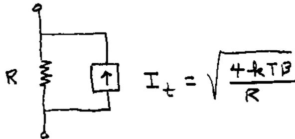
A resistor is the only passive element which can generate thermal noise. Capacitors and inductors do not generate thermal noise. We can prove this by contradiction. Assume a capacitor generates a noise  $V_{tc}$ . Connect it in parallel with a resistor which generates the noise  $V_{tr}$ . The circuit is as follows:
