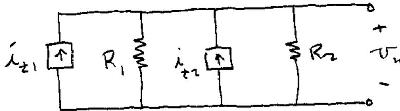
$$V_n = (i_{t1} + i_{t2}) \cdot R_1 \parallel R_2$$
