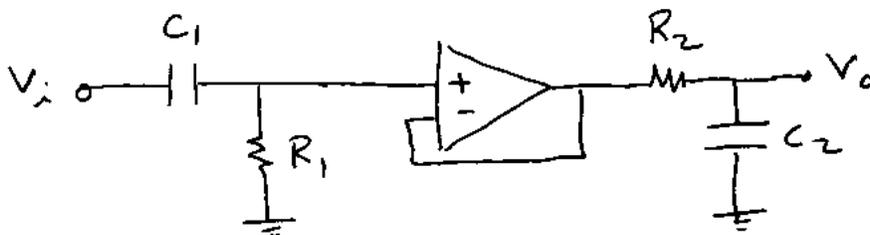
$$\frac{V_o}{V_i} = \frac{R_1 C_1 A}{1 + R_1 C_1 A} \times \frac{1}{1 + R_2 C_2 A}$$
