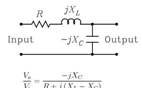
(b) The inductor is realized by a primarily inductive ferrite bead whose reactance is labeled "Bead 2" in the figure. Solve for the value of the capacitor such that the resonance frequency of the circuit is  $f_0 = 60 \,\mathrm{MHz}$ , i.e. the frequency at which  $X_L = X_C$ .
