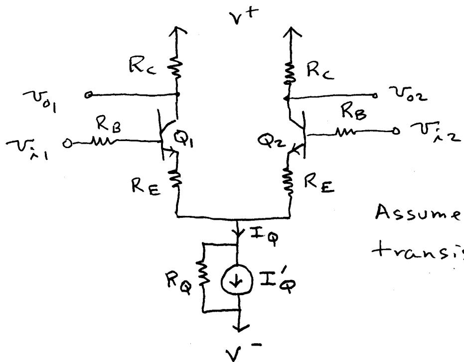
For the dc analysis, set  $v_{i1} = v_{i2} = 0$ . Divide the tail supply into 2 identical current sources ( $I_Q/2$  in parallel with  $2R_Q$ ). By symmetry the circuit for either  $Q_1$  or  $Q_2$
