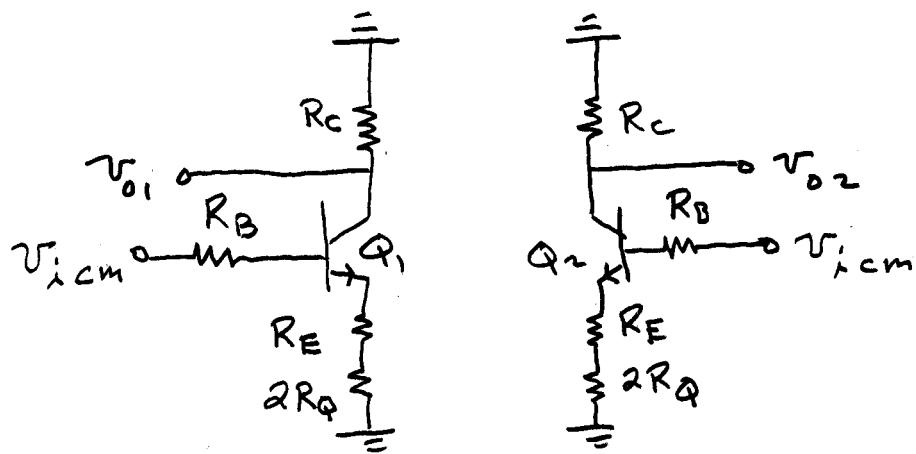
Thus the circuit again consists of two CE amplifiers. By symmetry,  $v_{o1} = v_{o2}$ . From our CE analysis, we have
