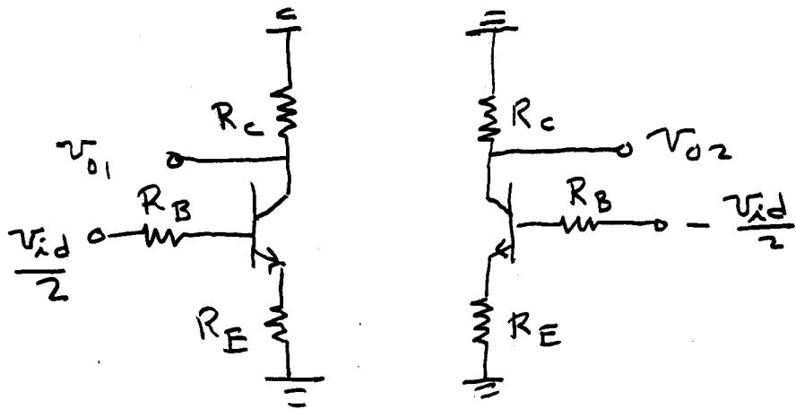
Thus the circuit consists of two CE amplifiers. By symmetry,  $v_{o2} = -v_{o1}$ . From our CE amplifier analysis, we have
