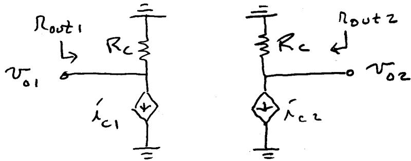
$$v_{o1} = -v_{o2} = -i_{c1} R_c = \frac{-\alpha R_c}{2(R'_e + R_E)} (v_{i1} - v_{i2})$$
