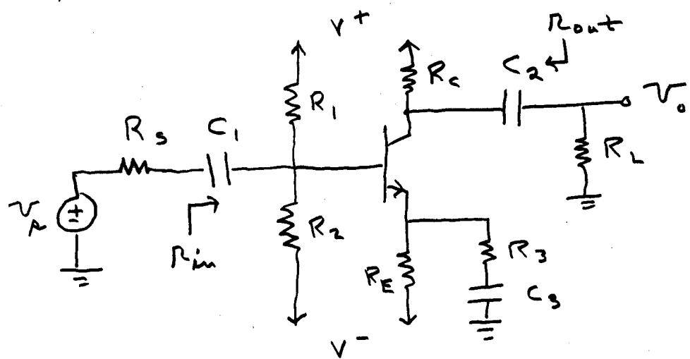
The dc bias currents and voltages are solved for assuming the capacitors are open circuits. For the ac small-signal solution, set  $v^+ = v^- = 0$  and assume the capacitors are ac short circuits. The circuit reduces to
