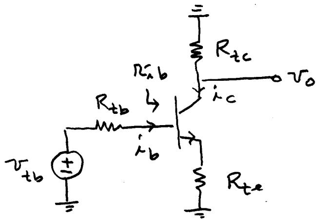
If  $r_x = 0$  and  $R_o = \infty$ ,  $R_{ib}$  is given by
