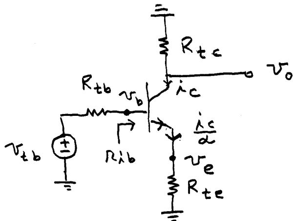
$$v_b = v_{tb} \frac{R_{ib}}{R_{tb} + R_{ib}} \quad v_e = \frac{i_c}{\alpha} R_{te}$$
