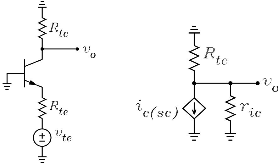
$$R_{tc} := R_P(R_C, R_L) \quad R_{tc} = 3.007 \cdot 10^3$$
