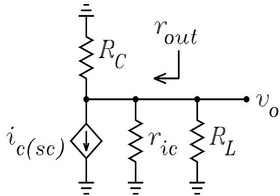
$$r_{out} := R_P(R_C, r_{ic}) \quad r_{out} = 4.263 \cdot 10^3$$
