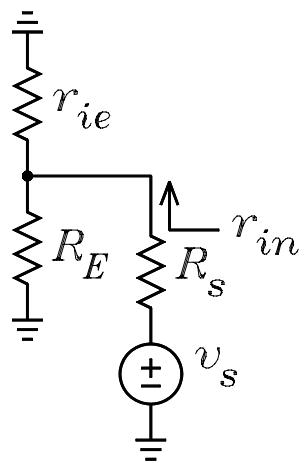
$$r_{ie} := r'_e \cdot \frac{r_0 + R_{tc}}{\frac{R_{tc}}{1 + \beta} + r_0 + r'_e} \quad r_{ie} = 10.569$$
