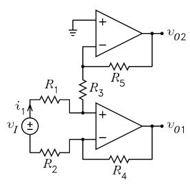
$$\begin{array}{lll} R_1 := 10000 & R_2 := 10000 & R_3 := 40000 & R_4 := 40000 & v_1 := 2 \\ i_1 := \frac{v_1}{R_1 + R_2} & i_1 = 1 \bullet 10^{-4} & v_{O1} := i_1 \cdot \left( R_3 + R_4 \right) & v_{O1} = 8 \\ \\ v_{O2} := -v_{O1} & R_5 := \frac{-v_{O2}}{i_1} & R_5 = 8 \bullet 10^4 \end{array}$$
