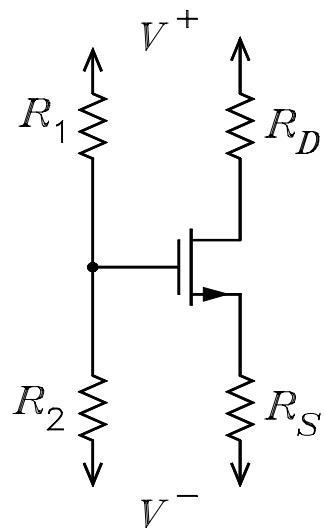
$$V_{GG} := \frac{V_{plus} \cdot R_2 + V_{minus} \cdot R_1}{R_1 + R_2} \quad V_{GG} = -16 \quad V_{SS} := V_{minus} \quad R_{SS} := R_S$$
