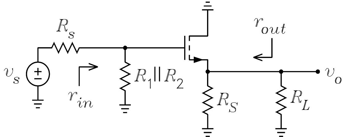
$$K := K_{\text{prime}} \cdot \frac{W}{L} \cdot (1 + \lambda \cdot V_{DS}) \quad K = 3.377 \cdot 10^{-3} \quad g_m := \sqrt{2 \cdot K \cdot I_D} \quad g_m = 3.343 \cdot 10^{-3}$$
