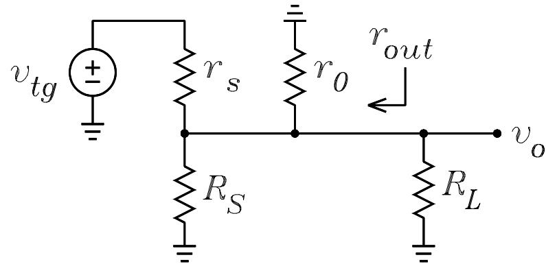
$$v_o := v_{tg} \cdot \frac{R_p(r_0, R_p(R_S, R_L))}{r_s + R_p(r_0, R_p(R_S, R_L))}$$
