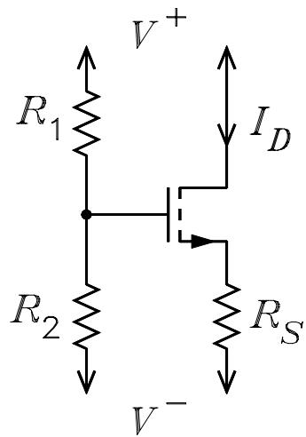
$$V_{GG} := \frac{V_{plus} \cdot R_2 + V_{minus} \cdot R_1}{R_1 + R_2} \quad V_{GG} = -16 \quad V_{SS} := V_{minus} \quad R_{SS} := R_S$$
