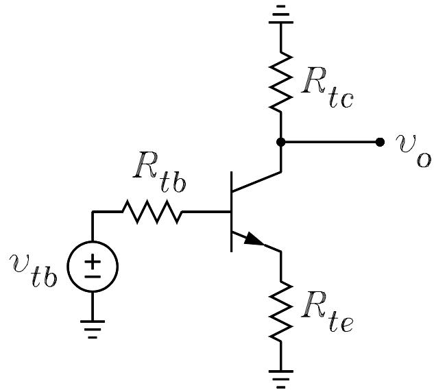
$$v_{tb} := v_s \cdot \frac{R_P(R_1, R_2)}{R_S + R_P(R_1, R_2)} \quad v_{tb} = 0.916 \quad R_{tb} := R_P(R_S, R_P(R_1, R_2)) \quad R_{tb} = 4.5802 \cdot 10^3$$
