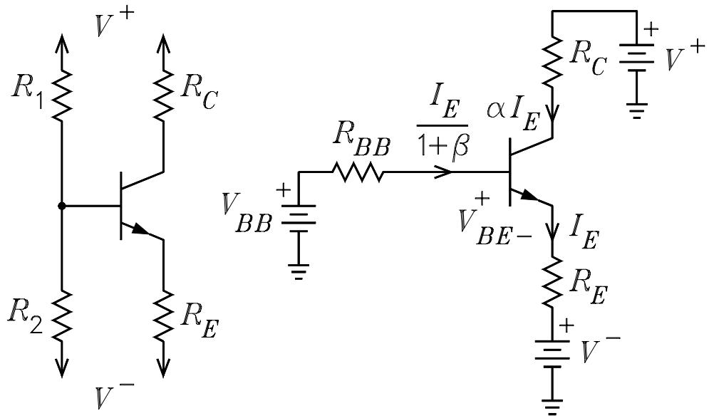
$$V_{BB} := \frac{V_p \cdot R_2 + V_m \cdot R_1}{R_1 + R_2} \quad V_{BB} = 1.3636 \quad R_{BB} := R_p(R_1, R_2) \quad R_{BB} = 5.4545 \cdot 10^4$$
