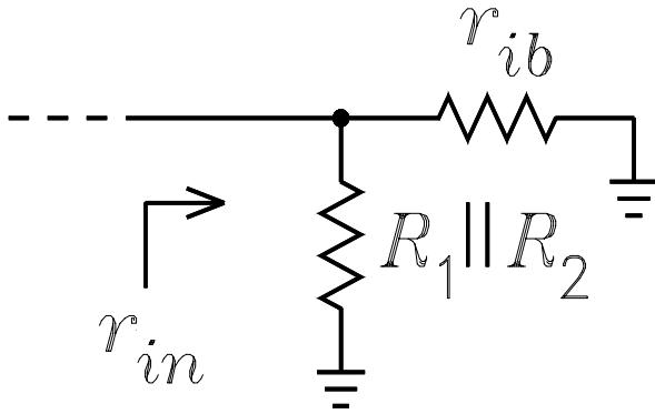
$$r_{ib} := r_x + r_\pi + (1 + \beta) \cdot R_{te}$$
