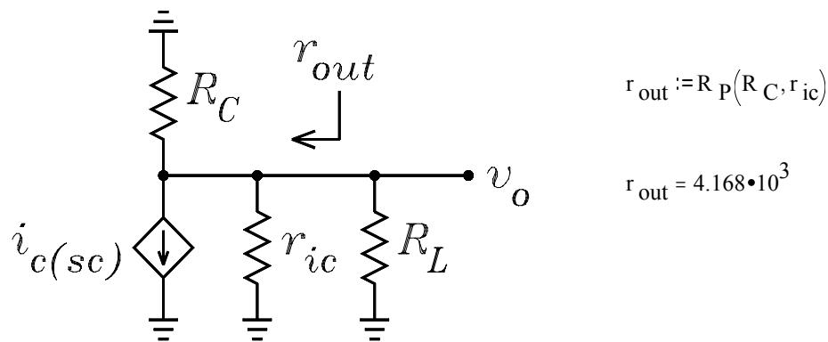
$$r_{out} := R_p(R_C, r_{ic})$$
