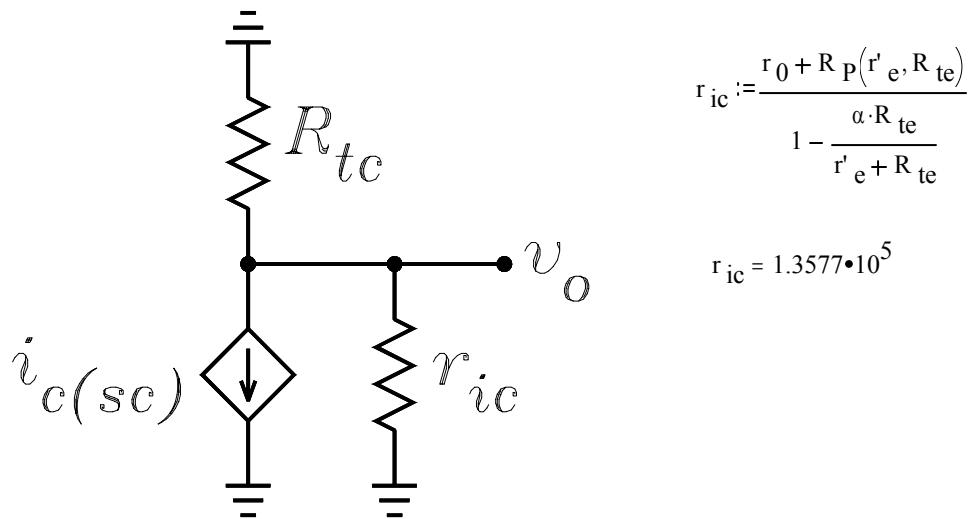
$$r_{ic} := \frac{r_0 + R_p(r'_e, R_{te})}{1 - \frac{\alpha \cdot R_{te}}{r'_e + R_{te}}}$$
