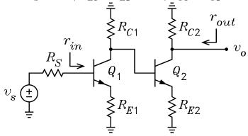
(a) Looking out of the base of  $Q_2$ , use the Norton collector circuit of  $Q_1$  to show that
