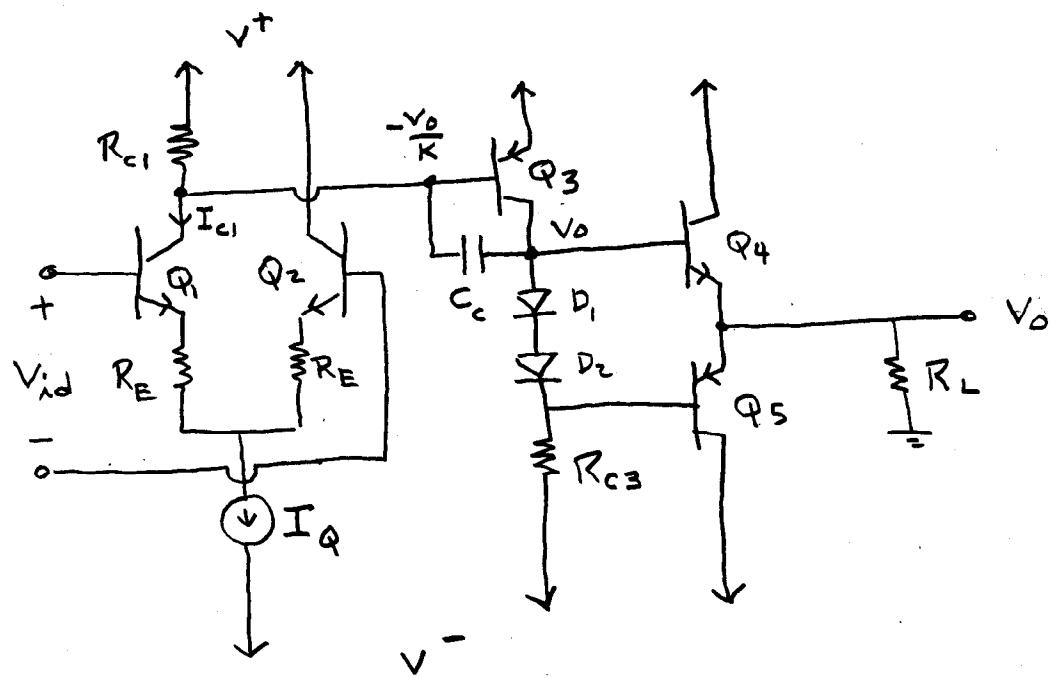
$Q_1$  and  $Q_2$  are a differential amplifier. We assume the current  $I_Q$  divides equally between  $Q_1$  and  $Q_2$  so that  $R_{E1} = R_{E2} = R_E = 2V_T/I_Q$ . For the analysis, we assume  $\alpha_1 = \alpha_2 = 1$ .
