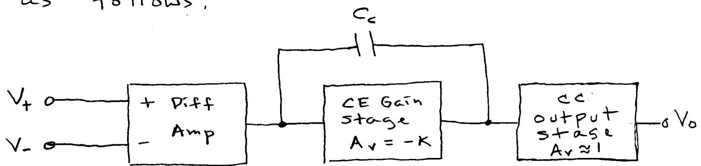
The diff amp subtracts the two input voltages to produce a difference voltage that drives a high gain stage which is usually a CE gain stage. The output stage is a complementary CC stage which supplies current gain to drive a load resistor.
