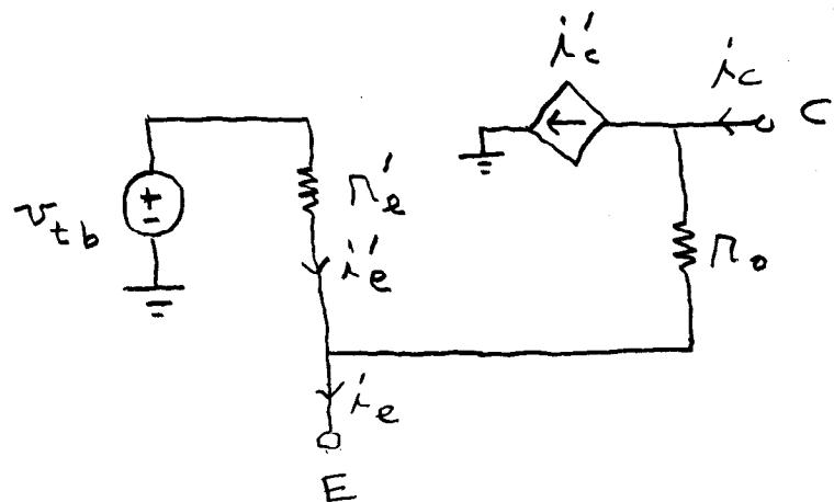
Note that the base node B has been absorbed. We use this model to solve the BJT differential amplifier.
