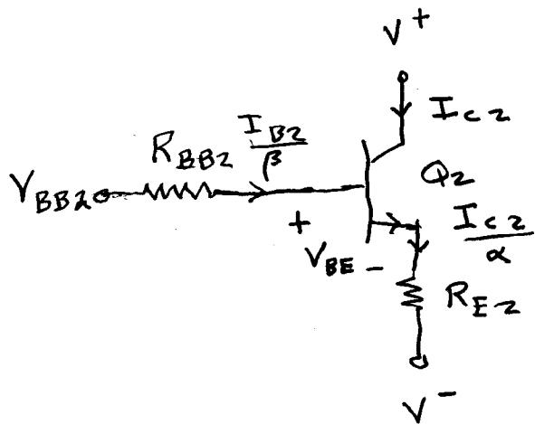
$$V_{BB2} - V^- = \frac{I_{C2}}{\beta} R_{BB2} + V_{BE} + \frac{I_{C2}}{\alpha} R_{E2}$$
