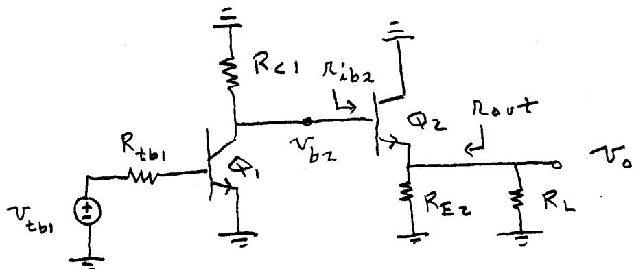
Note that  $r_{ib2}$  is the load resistor  $R_{L1}$  for  $Q_1$ . From our common-collector amplifier analysis, it is given by
