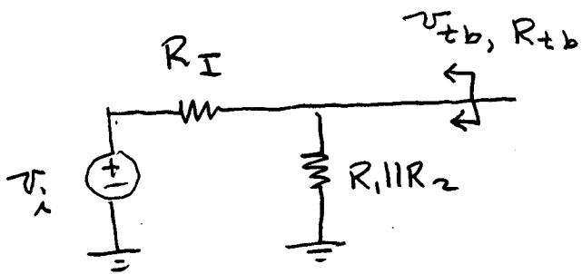
$$V_{tb} = V_i \frac{R_1 || R_2}{R_I + R_1 || R_2}$$
