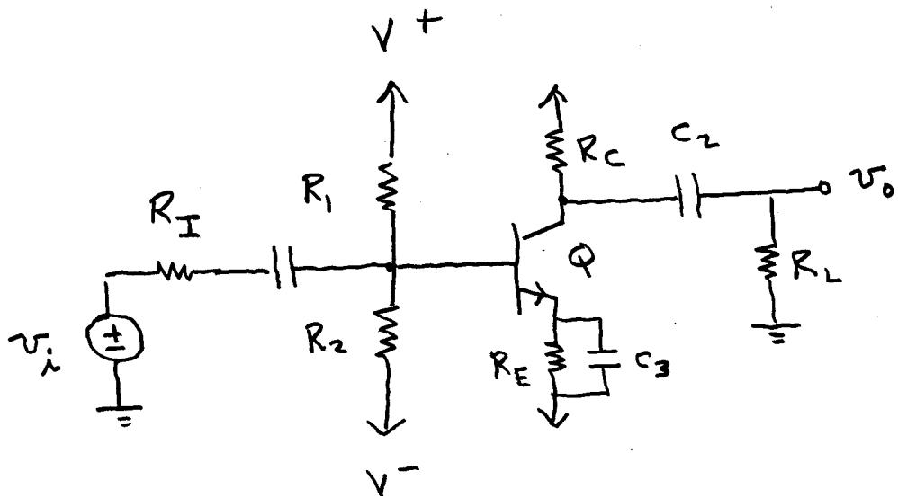
The Q point values are calculated with  $C_1$ ,  $C_2$ , and  $C_3$  open circuited. We assume this solution is known.
