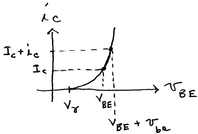
The Q point is  $(V_{BE}, I_c)$ . We wish to relate the small-signal change in  $I_c$  to the small-signal change in  $V_{BE}$ . The slope of the curve at the Q point is used to do this.
