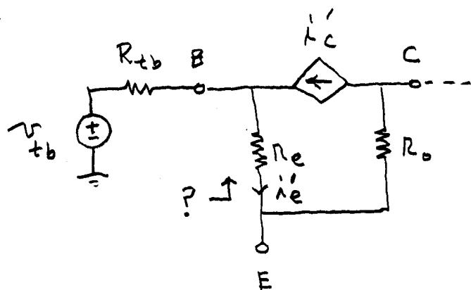
We wish to solve for the Thévenin equivalent circuit seen looking up into the  $i_e$  branch. The part of the circuit which we need for this
