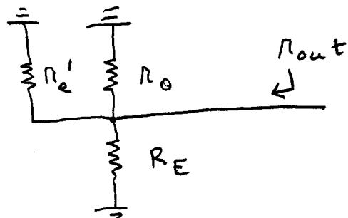
$$R_{out} = r'_e \parallel R_o \parallel R_E$$
