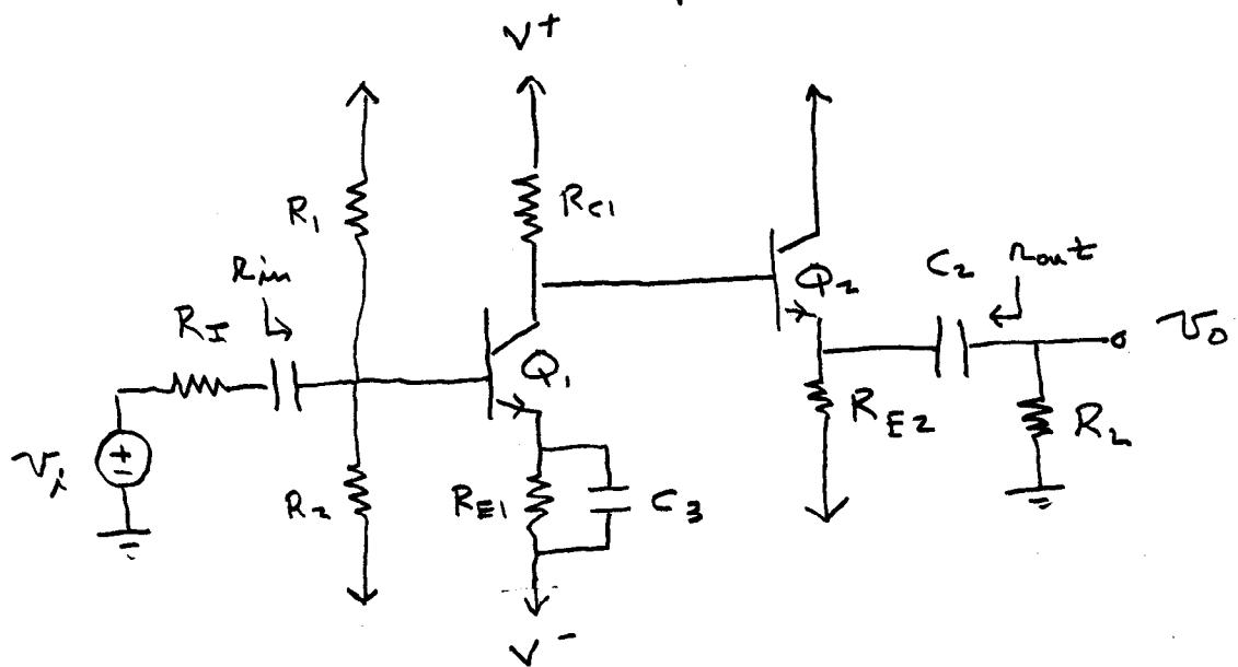
The dc bias solution for  $Q_1$  is the same as for the CE amp. The dc bias circuit for  $Q_2$  is
