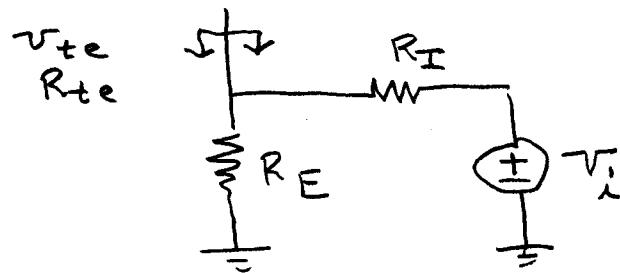
$$v_{te} = v_i \frac{R_E}{R_I + R_E} \quad R_{te} = R_E \parallel R_I$$
