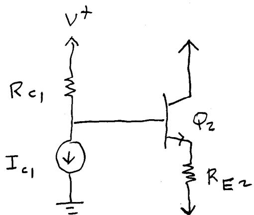
$$V_{BB2} = V^+ - I_{C1} R_{C1} \quad R_{BB2} = R_{C1}$$
