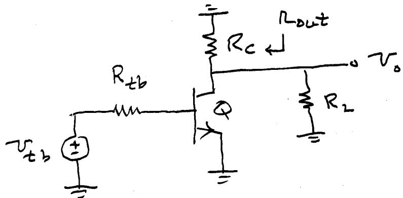
To solve for  $V_o$  and  $R_{out}$ , we replace  $Q$  with either the pi or the T model. Let us first use the pi model.
