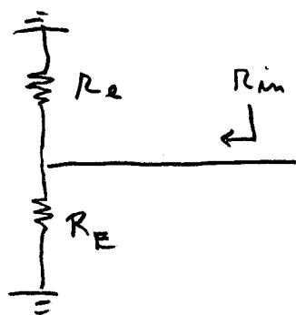
$$R_{in} = R_e \parallel R_E \quad R_e = \frac{V_T}{I_E}$$
