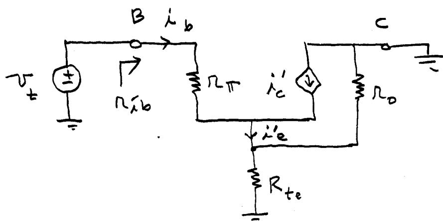
$$R_{ib} = \frac{V_t}{i_b}$$
