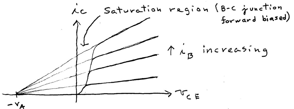
In the saturation region  $v_{CB} < 0$  so that  $v_{CE} = v_{CB} + v_{BE} < v_{BE}$ . That is  $v_{CE} < v_{BE}$ .
