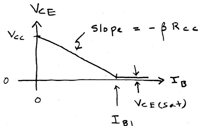
As  $I_B$  is increased,  $V_{CE}$  decreases, but it cannot go negative because the B-C junction becomes forward biased. When this happens,  $V_{CE}$  levels off at a value labeled
