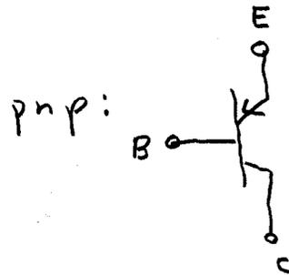
The leads are called the collector (C), the base (B), and the emitter E.
