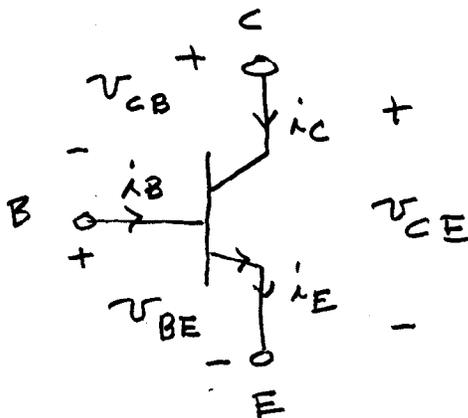
We will assume that the device is in its active mode and that the leakage currents can be neglected.
