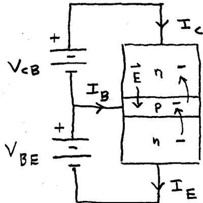
The battery  $V_{CB}$  reverse biases the collector-to-base junction. The battery  $V_{BE}$  forward biases the base-to-emitter junction. The two n regions are doped very heavily with n-type impurities. The p region is doped very lightly with a p-type impurity. Because of the way it is doped, the majority current carriers are free electrons.
