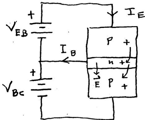
$V_{EB}$  forward biases the emitter-to-base junction.  $V_{BC}$  reverse biases the base-to-collector junction. The p-type regions
