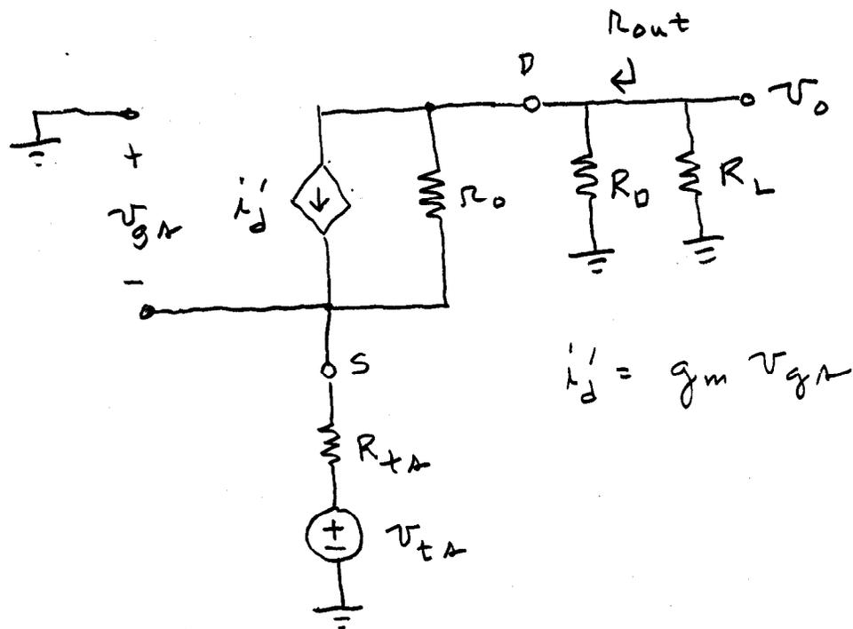
Note that neither end of  $R_o$  connects to ground. This greatly complicates the analysis. We will obtain an approximate solution by assuming the current through  $R_o$  can be neglected. That is, we let  $R_o = \infty$ .
