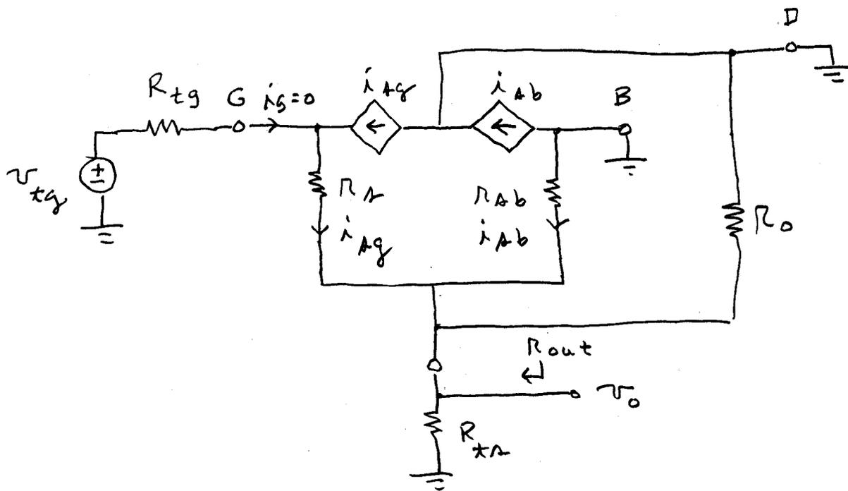
Set  $v_{xg} = 0$  to solve for  $R_{out}$ .
