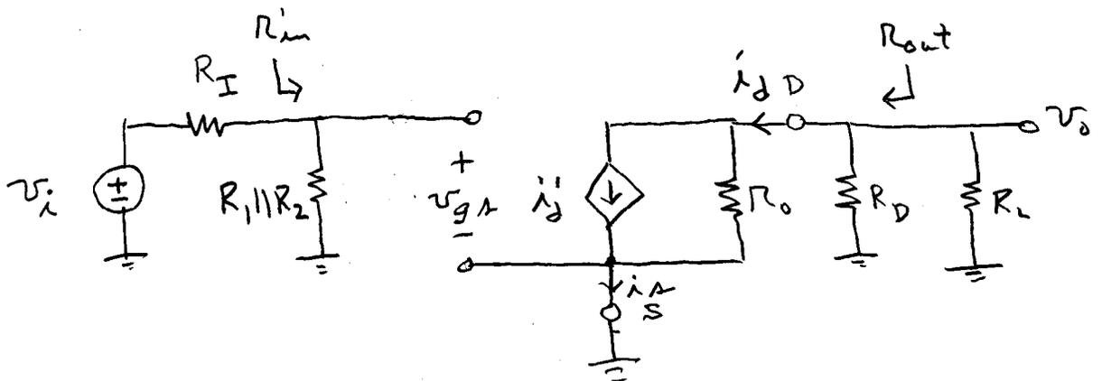
$$i'_d = g_m v_{gs} \quad g_m = 2\sqrt{K I_D}$$
