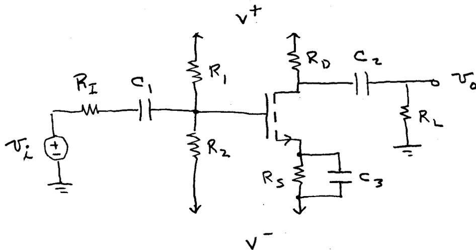
The Q point values are calculated with  $C_1$ ,  $C_2$ , and  $C_3$  open circuited. We assume this solution is known.
