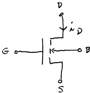
$$i_D = k (v_{GS} - V_{TH})^2$$
