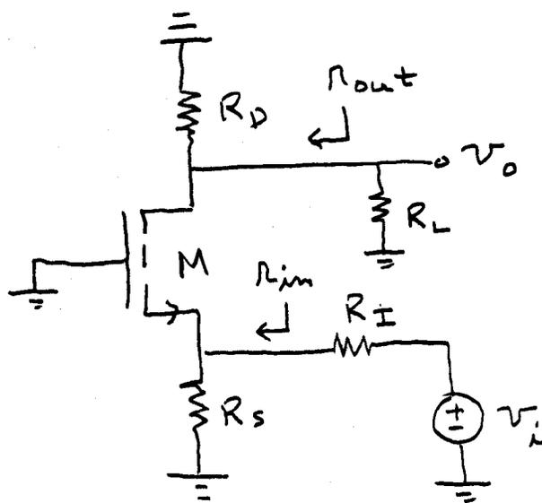
The solution for  $v_o$  and  $r_{out}$  is simplified by replacing the circuit looking out of the source by a Thévenin equivalent
