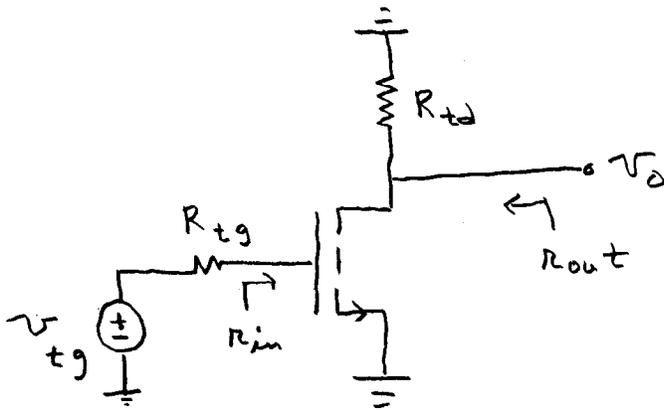
$$A_v = \frac{v_o}{v_{tg}} = -g_m (r_o \parallel R_{td})$$
