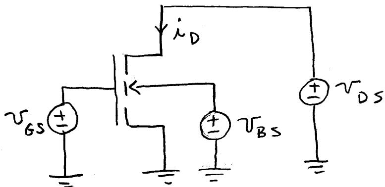
In this case, the threshold voltage is a function of  $V_{BS}$ . It is given by
