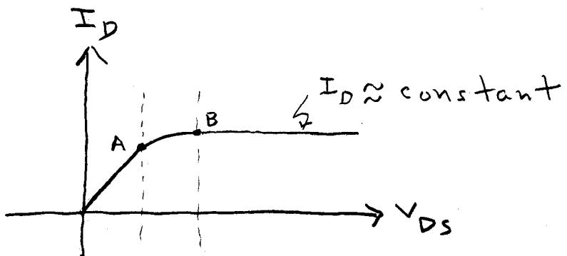
To the left of A, the device is not pinched off. The channel looks like a resistor. To the right of A, the device starts
