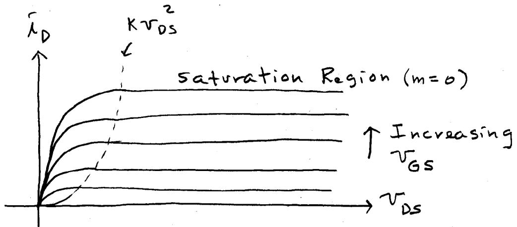
The plot of  $i_D$  versus  $V_{GS}$  is as follows
