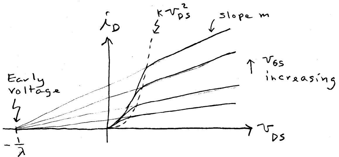
Because  $m = \frac{k'}{2} \frac{W}{L} \lambda (V_{GS} - V_{To})^2$ , it follows that the slope increases as  $V_{GS}$  increases.
