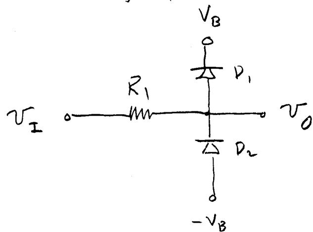
Replace the diodes with the large signal model
