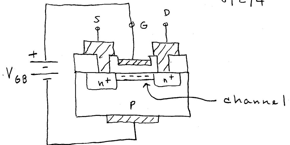
The region beneath the gate was a p region. Now it looks like an n region. It is called an inversion layer. It connects between the D and S. Mobile electrons can now travel from D to S if a voltage is applied between them.
