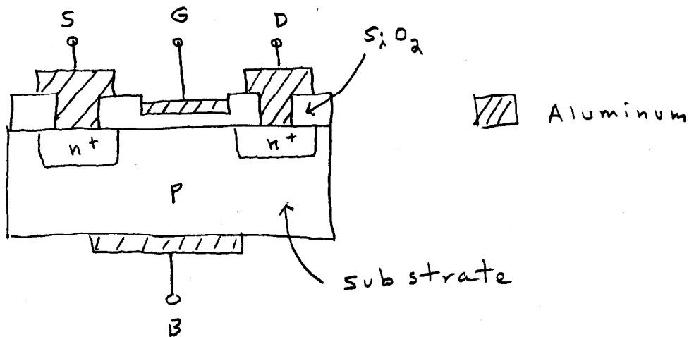
The SiO<sub>2</sub> between the Al contacts is an insulator.
