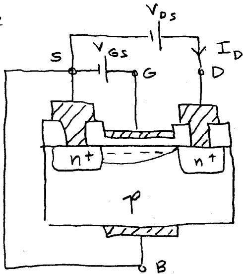
Assume  $V_{GS} > V_{TH}$ . For  $V_{DS} = 0$ , the inversion layer has a uniform thickness. As  $V_{DS}$  is increased, D pulls electrons from the inversion layer, causing its thickness to decrease at the end near the D. The figure shows the case where the thickness just goes to zero at the D region. The device is said to have reached pinch-off at point. If  $V_{DS}$  is increased further, we obtain
