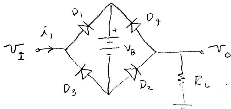
$$V_I > V_{D_1} + V_B + V_{D_2} \Rightarrow i_1 \text{ flows}$$
