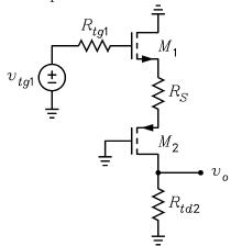
(a) Assume that  $r_0 = \infty$ . Replace the MOSFETs with the pi models and show that  $g_{m1}v_{gs1} = -g_{m2}v_{gs2}$ ,  $v_{tg1} = v_{gs1} + g_{m1}v_{gs1}R_S - v_{gs2}$ , and  $v_o = -g_{m2}v_{gs2}R_{td2}$ . Solve these equations to obtain
