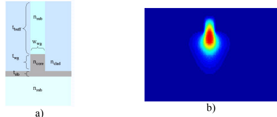
Figure 6: a) Rib waveguide geometry and b) field profile.
