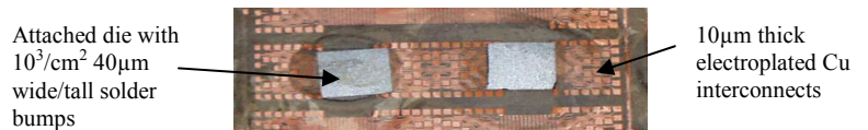
Fig. 10: A multi-crystalline Si board is used to fabricate a high-density substrate for SoL high-density packages. While organic substrates can also be used, this substrate is a potential alternative and its fabrication process is similar to that of on-chip multi-layer interconnect networks. The above micrograph shows two dice each with 10^3 area-array distribution of bumps on a \text{cm}^2 area bonded to the substrate. The dark region around the dice is flux residue.
