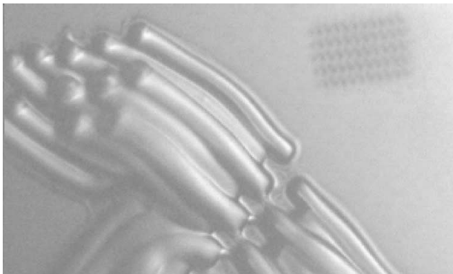
Fig. 13. Micrograph of a set of 100\text{-}\mu\text{m} tall and 10\text{-}\mu\text{m} wide circular polymer pillars after spray developing. Clearly, while the pillars were resolved, the very high aspect ratio polymer pillars were mechanically unstable and thus, collapsed.
