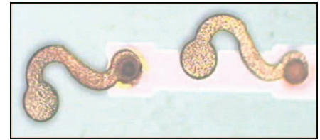
Figure 4. Micrograph showing slippery leads fabricated using Method 1 described in Figure 3 (i.e., using an Au seed layer). The lead on the left has moved by approximately 70 \mu\text{m} after the application of a lateral force.
