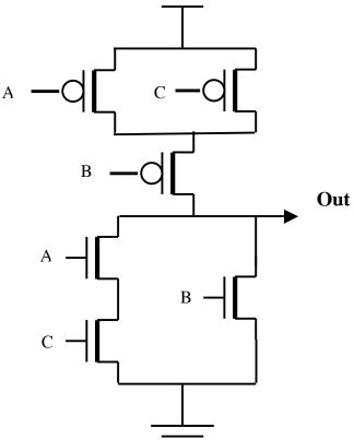
Write the Boolean expression for this function  $\underline{pmos} \rightarrow \underline{B'(A'+C')} \underline{nmos} \rightarrow (\underline{AC+B})'$
