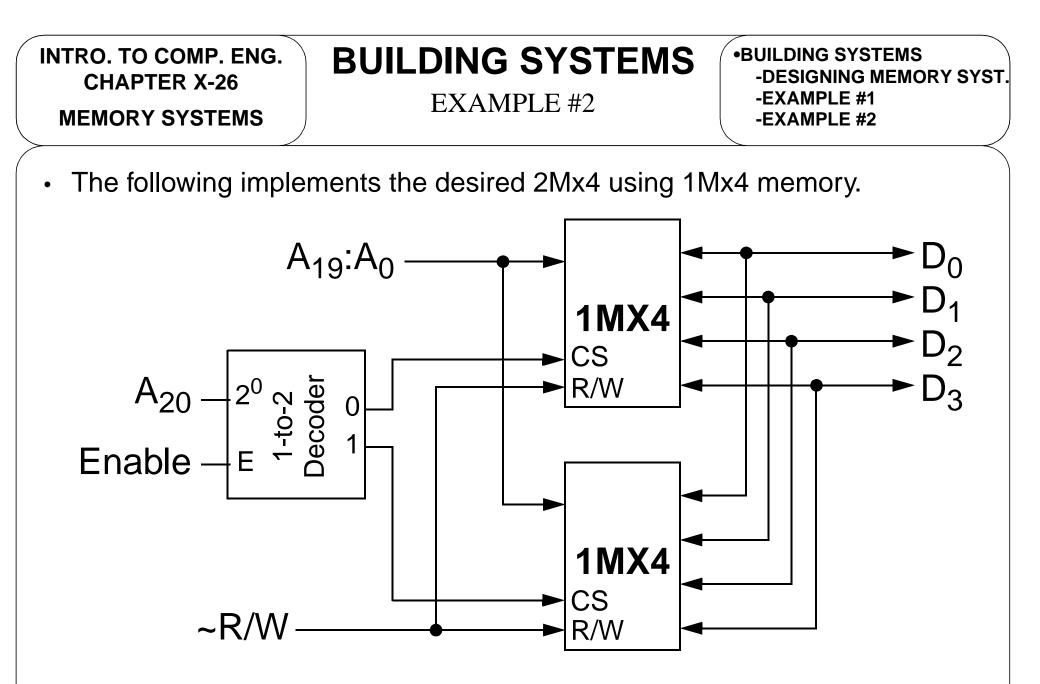
• Notice that A<sub>20</sub> is used to activate one of the **1Mx4** memory chips.
