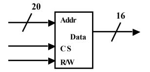
C. Show how to connect these  $1M \ge 16$  chips to make a 2M by 16 memory. The data outputs are three-state bus drivers.
